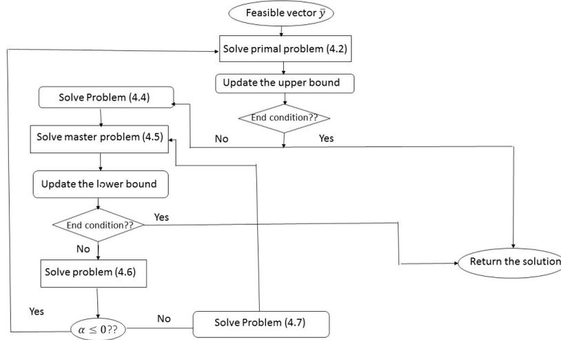
Figure 1: The overall framework of the proposed algorithm
